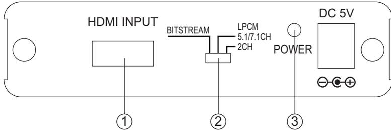
1. HDMI input: Connect the HDMI input port to the HDMI output port of your source equipment such as DVD player or set-top-box.
