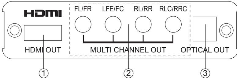
1. HDMI output: Connect the HDMI output port to the HDMI input port of your display.
